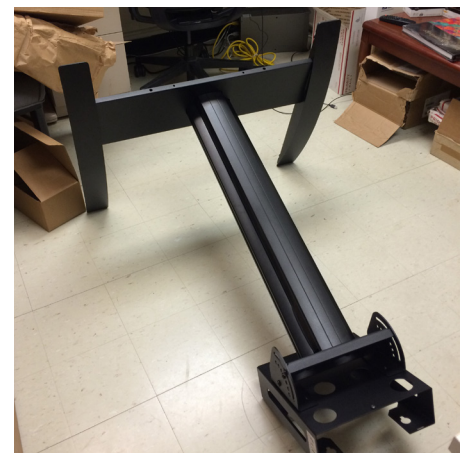
Fig. 3.2 - Attaching base to upright
